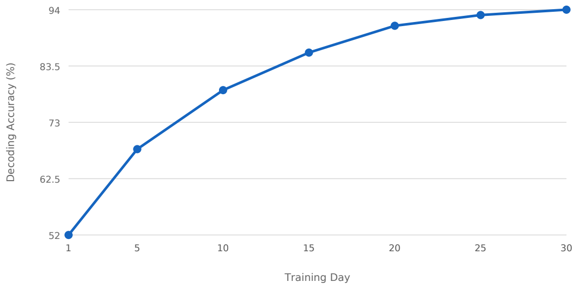
Figure 2. Motor decoding accuracy (% correct) for 2D cursor control using HD-MEA neural signals with a Kalman filter decoder
